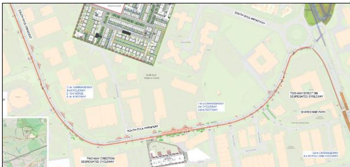
Figure 4 –South Gyle Crescent: two-way segregated cycle track and improved public space
